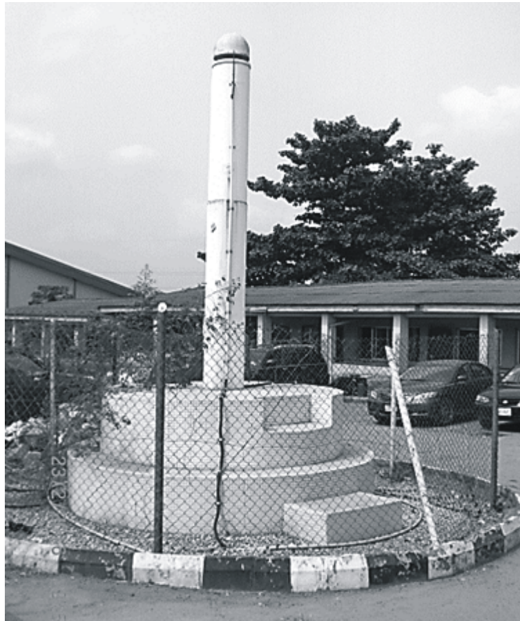
Fig. 3: The CORS located at the Lagos State Surveyor-General's office, Alausa, Ikeja
